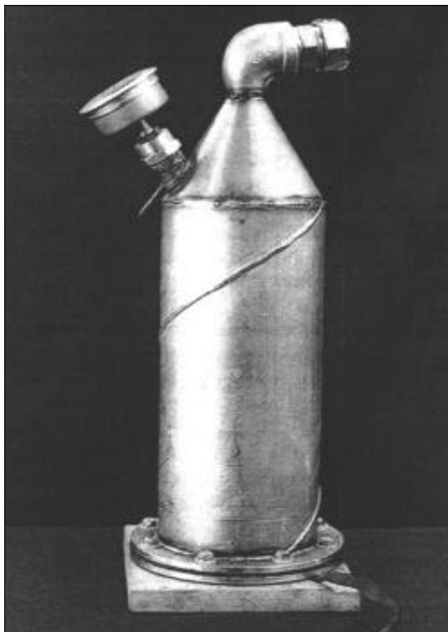
Fig. 1: A view of "Old Trusty", a three-year-old cell that breaks most of the rules of cell design, but is still a great performer. The filling hole has a temporary pressure gauge fitted to monitor air leaks.
